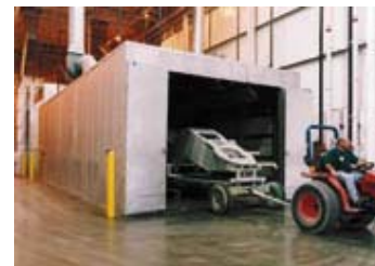
A 6,000 lb hydraulic crane upper frame is removed from the catalytic infrared curing oven for cool down.
