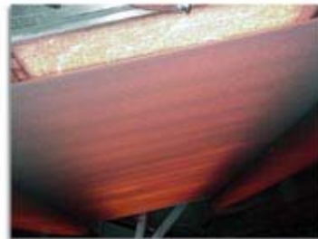
Gas infrared emitters are used to dry and cure coatings on paper and other web-based products.
