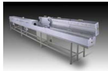
Figure 4. This oven dries and cures a solvent-based adhesive coating that is applied to both sides of a narrow steel strip. It combines hot air for solvent drying and lower explosive limit (LEL) control with infrared heat for drying and curing.
