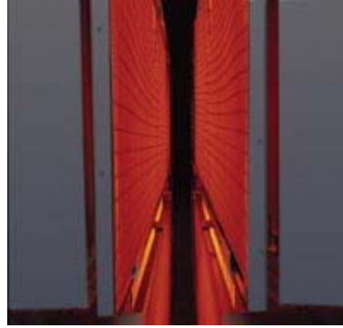
Figure 3. This vertical dual-radiation electric infrared tower preheats a paper web to reduce residual moisture before a urethane coating is applied. Electric infrared heaters on both sides of the product deliver massive amounts of energy while an optical pyrometer control maintains exact temperature in the system.
