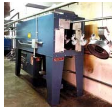
This combination convection/infrared oven cures powder on aluminum castings with complex shapes.
