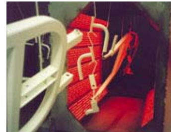
Figure 2. Infrared ovens can gel a powder coating on an assembly of parts with varying masses and cross-sections.
