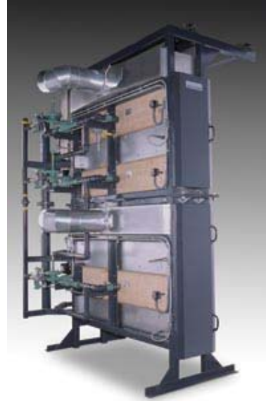
Figure 4. This vertical gas infrared fabric predryer blasts the product with high intensity infrared energy from both sides, which helps to kick off the drying process and allows faster line speeds.
