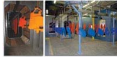
Figure 2. Modern manufacturing trends demand a highly flexible curing system that can handle a range of product sizes on the same curing line. Here, a light gauge part exits the oven's infrared booster while a heavy part enters it (left). Heavier items can be run down the finishing line at the same production rate as lighter items (right).
