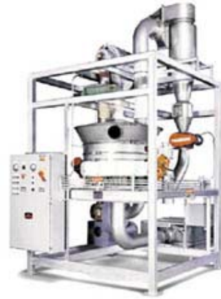
This 48" dia. fluid bed dryer reduces moisture content of 50 micron mesh size ceramic particles from 7 percent to 2 percent at a continuous rate of 1,000 lb/hr.
