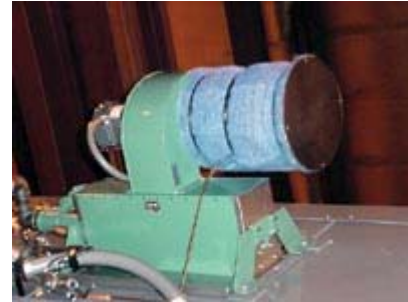
Figure 2. A combustion filter is a low-cost item that will keep the burner clean and operating at peak efficiency.
