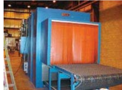
Figure 1. Profile curtains seal the area above a conveyor but let the product pass through, resulting in reduced heat losses out the openings.
