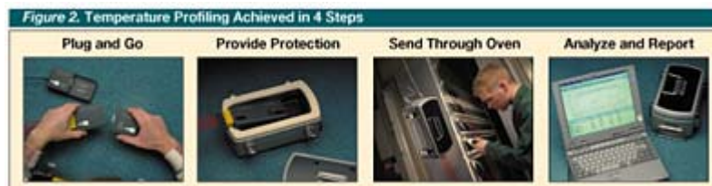
Figure 2. Temperature profiling can be accomplished in four simple steps: connect datalogger and transducer, place in thermal barrier, send through oven, and analyze and report results.
