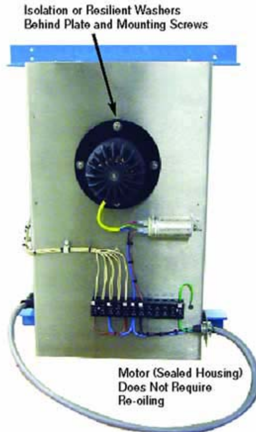
Figure 2. This ball-bearing motor does not require periodic re-oiling; instead, this type of motor normally has a sealed housing.
