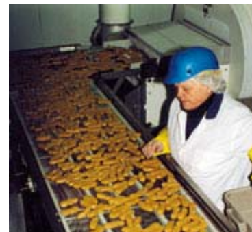
A quality control inspector at D.C. Foods examines parfried breaded chicken strips as they leave the Meyn fryer. During frying, the cooking oil's temperature is maintained within 11°C.
