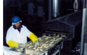
At D.C. Foods, uncooked breaded chicken strips are placed on flat, nonstick bars that carry the product through the Meyn fryer for processing. The fryer is heated by a Fulton thermal fluid heater filled with Paratherm NF heat transfer fluid.
